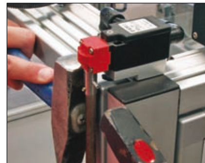
Switch locking (pin provided).
