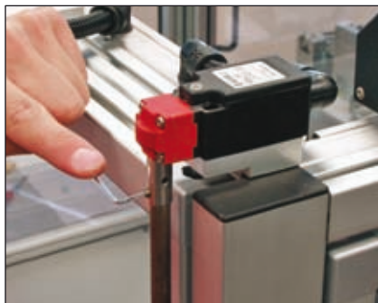
Temporary shaft locking (dowel provided).
